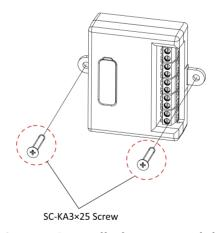
Figure 4-2 Install Alarm In Module
