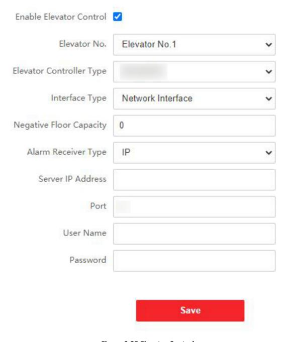
**Figure 6-25 Elevator Control**
