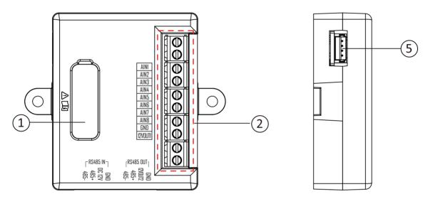
Figure 2-1 Alarm In Module
