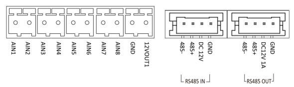
**Figure 3-1 Alarm In Module Terminals**
