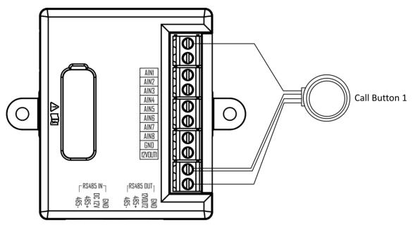
Figure 3-2 Call Button Wiring
